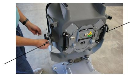
Figure 32: Removing Screws from Yoke Safety Bars
