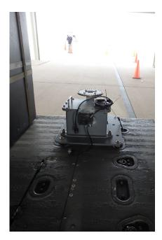
Figure 24: Placing Mounting Plate and Battery Box into Aircraft (BACK)
