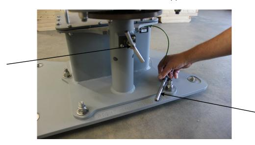
Figure 34: Friction Lock T-Handle (left) and Stud Safety Pin (right)
