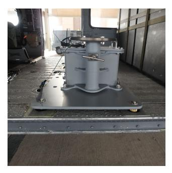
Figure 23: Placing Mounting Plate and Battery Box into Aircraft (FRONT)
