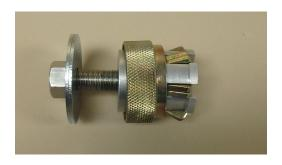
Figure 26: 12-Jaw Cargo Fitting Example
